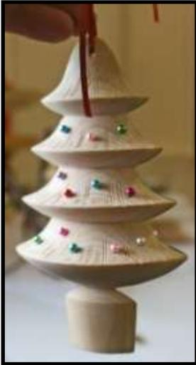
Starting from the widest point cut in with a spindle gouge to form the tree shape. It is important that everything was central at the start as any discrepancy will now begin to show. Finally form the base or pot and then abrade through the grits.
